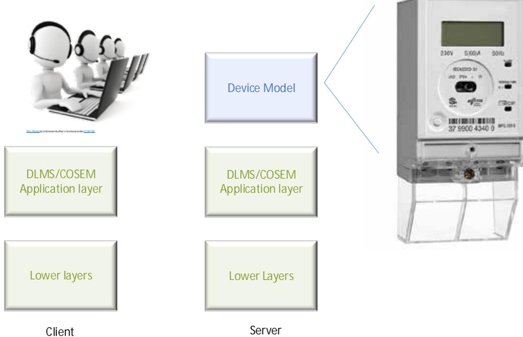
**Figure 1 – DLMS Architecture**
