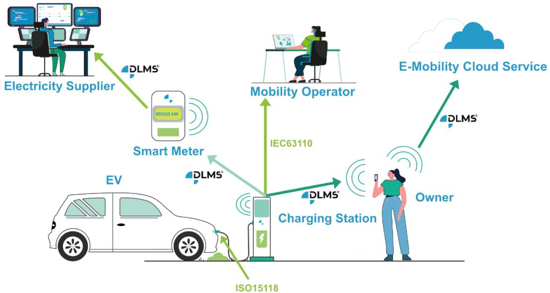
Figure 2 - EV Charging provided by an EV Mobility Operator
